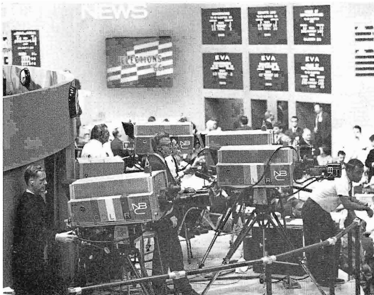
Election Night at NBC was "crucible of color technology" for these massed TK-43 cameras.
