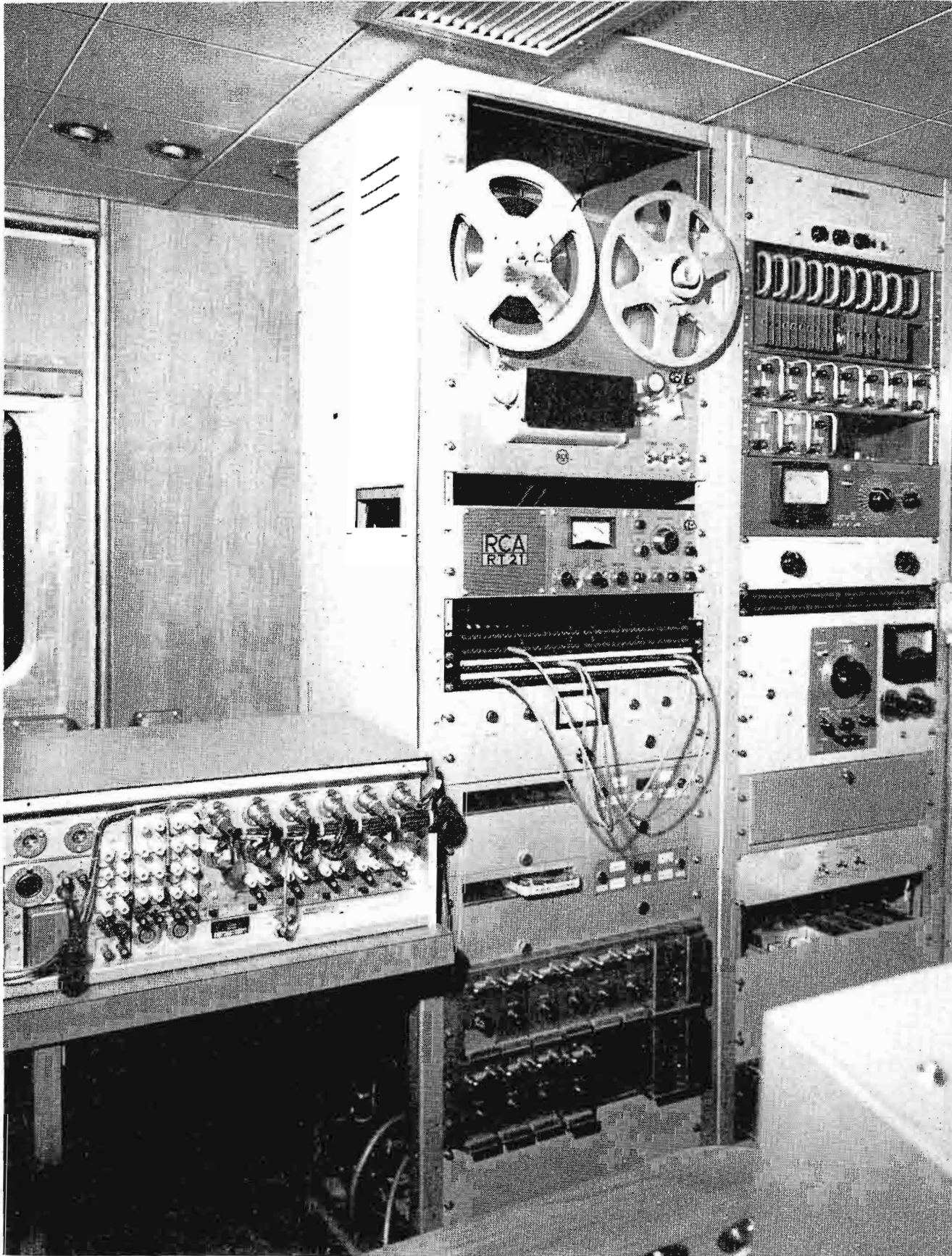
FIG. 11. The main audio racks: illustrating RT-21 reel-to-reel tape, and two cartridge tape units (1 record and replay, and 1 replay only.)
